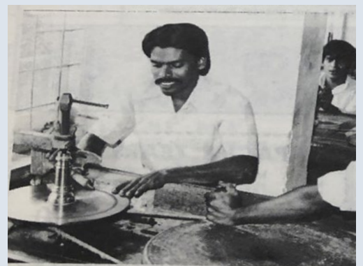
Traditional gem faceter using Wadi polishing abrasive
